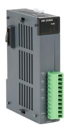
LS Electric XGB analog output module, 4-channel, voltage, 12-bit, output voltage signal range(s) of 0-10 VDC, external 24 VDC required.
