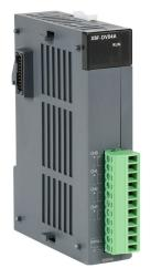
LS Electric XGB analog output module, 4-channel, voltage, 12-bit, output voltage signal range(s) of 0-10 VDC, external 24 VDC required.
