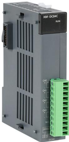
LS Electric XGB analog output module, 4-channel, current, 14-bit, output current signal range(s) of 0-20 mA and 4-20 mA, external 24 VDC required.
