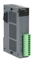
LS Electric XGB analog output module, 4-channel, current, 12-bit, output current signal range(s) of 0-20 mA and 4-20 mA, external 24 VDC required.
