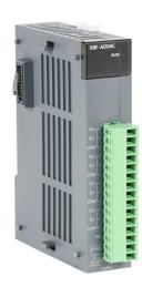
LS Electric XGB analog input module, 4-channel, current/voltage, 14-bit, input current signal range(s) of 0-20 mA, 4-20 mA, input voltage signal range(s) of 0-5 VDC, 1-5 VDC, 0-10 VDC, +/-10 VDC, external 24 VDC required.
