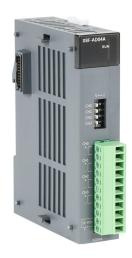
LS Electric XGB analog input module, 4-channel, current/voltage, 12-bit, input current signal range(s) of 0-20 mA, 4-20 mA, input voltage signal range(s) of 0-10 VDC, external 24 VDC required.
