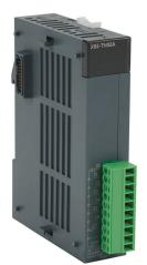
LS Electric XGB discrete output module, 8-point, 12-24 VDC, sinking, 1 common(s), 8 point(s) per common, 0.5A/point, 2A/ common. Removable terminal blocks included.
