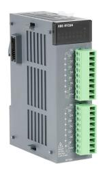
LS Electric XGB relay output module, 16-point, 125 VDC/250 VAC, (16) Form A, 2 isolated common(s), 8 point(s) per common, 2A/point, 5A/common. Removable terminal blocks included.
