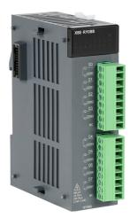
LS Electric XGB relay output module, 8-point, 125 VDC/250 VAC, (8) Form A, 8 isolated common(s), 1 point(s) per common, 2A/ point. Removable terminal blocks included.
