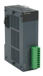
LS Electric XGB relay output module, 8-point, 125 VDC/250 VAC, (8) Form A, 1 common(s), 8 point(s) per common, 2A/point, 5A/common. Removable terminal block included.
