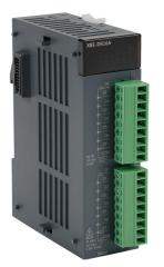
LS Electric XGB discrete combo module, Input: 8-point, 24 VDC, sinking/sourcing, Output: 8-point, 125 VDC/250 VAC, relay, (8) Form A (SPST) relays, 2A/point, 5A/common. Removable terminal blocks included.
