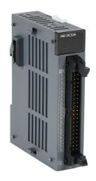
LS Electric XGB discrete input module, 32-point, 24 VDC, sinking/sourcing, 1 common(s), 32 point(s) per common. Requires XTB-40H terminal block and C40HH-xxSB-XBI cable.
