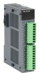
LS Electric XGB discrete input module, 16-point, 24 VDC, sinking/ sourcing, 1 common(s), 16 point(s) per common. Removable terminal blocks included.
