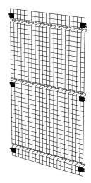
Velox machine guarding panel, 66 x 40in, 2 x 2in grid, 8 gauge wire, carbon steel, black.
