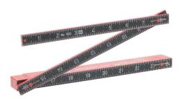
Wiha MaxiFlex series folding ruler, 6.5ft/2m length, metric inside and imperial outside reading, 1/16in and 1mm marks, 10 sections, 0, 90, and 180 degree lock-in-place stop-joints.
