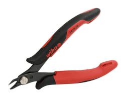
Wiha precision diagonal full flush cutters, 5.0in (127mm) overall length, ultra full flush cutting edge, 21 degrees angled head, electronic cushion grip handles.
