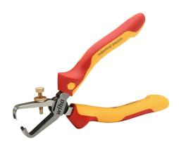
Wiha wire stripping pliers, 6.3in (160mm) overall length, insulated, 1000V insulation rating, induction hardened beveled cutting edges, insulated cushion grip handles.
