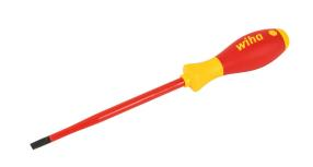
Wiha SlimLine 6.5mm slotted insulated screwdriver, 1000V insulation rating, 5.9in (150mm) shaft length, reduced shank, SoftFinish cushion grip handle.
