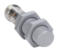
AutomationDirect inductive proximity sensor, tubular, 12mm diameter x 45mm body, weld coated 316 stainless steel housing, PNP, N.O. output, 4mm sensing distance, flush, 2 Hz switching frequency, IP65 IP66 IP67 IP68 IP69K, 4-pin M12 quick-disconnect.
