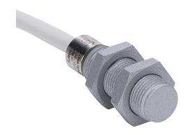
AutomationDirect inductive proximity sensor, tubular, 12mm diameter x 40mm body, weld coated 316 stainless steel housing, NPN/PNP, N.O. output, 4mm sensing distance, flush, 75 Hz switching frequency, IP67, 4-pin M12 quick-disconnect.
