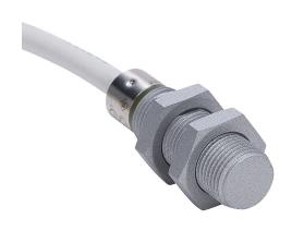
AutomationDirect inductive proximity sensor, tubular, 12mm diameter x 40mm body, weld coated 316 stainless steel housing, NPN/PNP, N.O. output, 4mm sensing distance, flush, 75 Hz switching frequency, IP67, pigtail.
