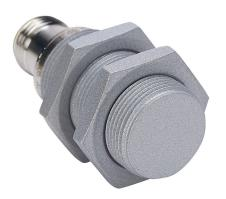
AutomationDirect inductive proximity sensor, tubular, 18mm diameter x 45mm body, weld coated 316 stainless steel housing, PNP, N.O. output, 8mm sensing distance, flush, 2 Hz switching frequency, IP65 IP66 IP67 IP68 IP69K, 4-pin M12 quick-disconnect.
