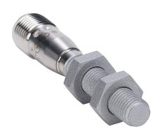
AutomationDirect inductive proximity sensor, tubular, 8mm diameter x 60mm body, weld coated 316 stainless steel housing, PNP, N.O. output, 2mm sensing distance, flush, 100 Hz switching frequency, IP67 IP68, 4-pin M12 quick-disconnect.
