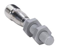
AutomationDirect inductive proximity sensor, tubular, 8mm diameter x 60mm body, weld coated 316 stainless steel housing, PNP, N.O. output, 2mm sensing distance, flush, 100 Hz switching frequency, IP67 IP68, 4-pin M12 quick-disconnect.
