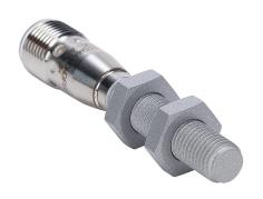
AutomationDirect inductive proximity sensor, tubular, 8mm diameter x 60mm body, weld coated 316 stainless steel housing, NPN, N.O. output, 2mm sensing distance, flush, 100 Hz switching frequency, IP67 IP68, 4-pin M12 quick-disconnect.
