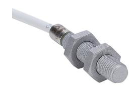
AutomationDirect inductive proximity sensor, tubular, 8mm diameter x 45mm body, weld coated 316 stainless steel housing, NPN/PNP, N.O. output, 2mm sensing distance, flush, 150 Hz switching frequency, IP67, 4-pin M12 quick-disconnect.
