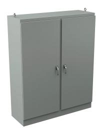
Wiegmann KwikHinge series enclosure, NEMA 3R/4/12, 90 x 72 x 24in (HxWxD), freestanding, carbon steel, ANSI 61 gray, powder coat finish, 2-door, 3-point keylocking/padlocking combo handle.
