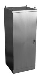
Wiegmann KwikHinge series enclosure, NEMA 3R/4/4X/12, 90 x 36 x 36in (HxWxD), freestanding mount, 304 stainless steel, No. 3 intermediate polished finish, single-door, 3-point keylocking/padlocking combo handle.
