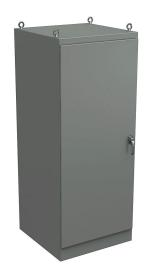
Wiegmann KwikHinge series enclosure, NEMA 3R/4/12, 90 x 36 x 36in (HxWxD), freestanding, carbon steel, ANSI 61 gray, powder coat finish, single-door, 3-point keylocking/padlocking combo handle.
