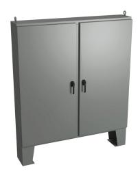
Wiegmann KwikHinge series enclosure, NEMA 3R/4/12, 74 x 72 x 12in (HxWxD), floor mount, carbon steel, ANSI 61 gray, powder coat finish, 2-door, 3-point keylocking/padlocking combo handle.
