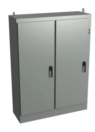
Wiegmann KwikHinge series disconnect enclosure, NEMA 3R/4/12, right flange, 72 x 53 x 18in (HxWxD), freestanding, carbon steel, ANSI 61 gray, powder coat finish, 2-door, 3-point keylocking/padlocking combo handle, subpanel included.
