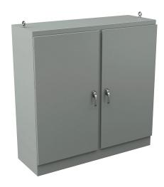
Wiegmann KwikHinge series enclosure, NEMA 3R/4/12, 72 x 72 x 24in (HxWxD), freestanding, carbon steel, ANSI 61 gray, powder coat finish, 2-door, 3-point keylocking/padlocking combo handle.
