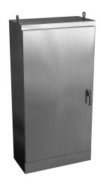
Wiegmann KwikHinge series enclosure, NEMA 3R/4/4X/12, 72 x 36 x 18in (HxWxD), freestanding mount, 304 stainless steel, No. 3 intermediate polished finish, single-door, 3-point keylocking/padlocking combo handle.
