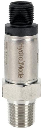
HydroMode pressure transmitter, 0 to 150 psig range, +/- 1% accuracy, stainless steel sensing element, 4-20 mA analog output, 1/4in male NPT process connection, 8-32 VDC operating voltage, 4-pin M12 quick-disconnect, NSF/ANSI/CAN 61 and NSF 372.
