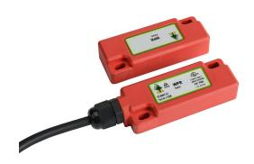
IDEM safety switch set, non-contact magnetic, (2) N.C. safety output(s), (1) N.O. monitoring output(s), plastic housing, 75 x 29mm, 8-pin M12 quick-disconnect, 9.8in/250mm cable length.
