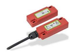
IDEM safety switch set, non-contact magnetic, (2) N.C. safety output(s), (1) N.O. monitoring output(s), plastic housing, 75 x 29mm, pigtail, 6.5 ft/2m cable length.
