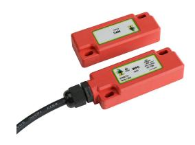
IDEM safety switch set, non-contact coded magnetic, (2) N.C. safety output(s), (1) N.O. monitoring output(s), plastic housing, 75 x 29mm, 8-pin M12 quick-disconnect, 9.8in/250mm cable length.
