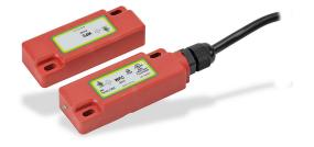
IDEM safety switch set, non-contact coded magnetic, (2) N.C. safety output(s), (1) N.O. monitoring output(s), plastic housing, 75 x 29mm, pigtail, 16.4ft/5m cable length.
