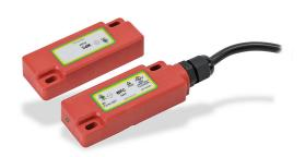
IDEM safety switch set, non-contact coded magnetic, (2) N.C. safety output(s), (1) N.O. monitoring output(s), plastic housing, 75 x 29mm, pigtail, 6.5ft/2m cable length.
