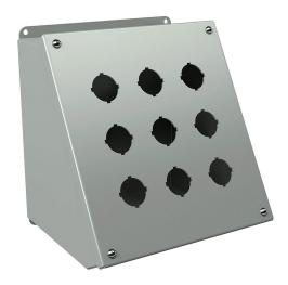
Wiegmann pushbutton consolet, 9 holes, 30mm, NEMA 12/13, 10 x 9 x 8in (HxWxD), wall mount, carbon steel, ANSI 61 gray, powder coat finish, screw cover.
