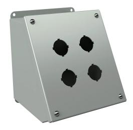
Wiegmann pushbutton consolet, 4 holes, 30mm, NEMA 12/13, 7 x 6 x 7in (HxWxD), wall mount, carbon steel, ANSI 61 gray, powder coat finish, screw cover.
