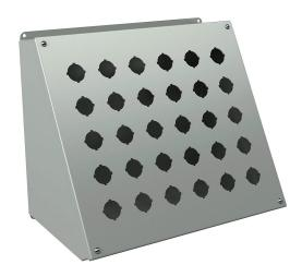
Wiegmann pushbutton consolet, 30 holes, 30mm, NEMA 12/13,  $14 \times 15 \times 10$  in (HxWxD), wall mount, carbon steel, ANSI 61 gray, powder coat finish, screw cover.
