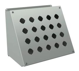
Wiegmann pushbutton consolet, 20 holes, 30mm, NEMA 12/13, 12 x 13 x 9in (HxWxD), wall mount, carbon steel, ANSI 61 gray, powder coat finish, screw cover.
