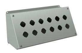
Wiegmann pushbutton consolet, 12 holes, 30mm, NEMA 12/13, 7 x 15 x 7in (HxWxD), wall mount, carbon steel, ANSI 61 gray, powder coat finish, screw cover.
