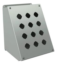
Wiegmann pushbutton consolet, 12 holes, 30mm, NEMA 12/13, 12 x 9 x 9in (HxWxD), wall mount, carbon steel, ANSI 61 gray, powder coat finish, screw cover.
