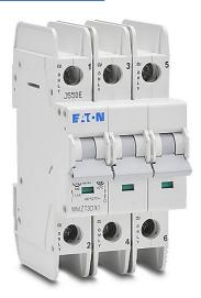
Eaton miniature circuit breaker, current-limiting, 1.5A, 480Y/277 VAC/96 VDC, 3-pole, D curve, thermal magnetic, 35mm DIN rail mount.
