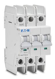
Eaton miniature circuit breaker, current-limiting, 4A, 480Y/277 VAC/96 VDC, 3-pole, D curve, thermal magnetic, 35mm DIN rail mount.
