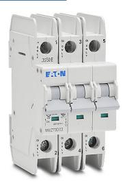
Eaton miniature circuit breaker, current-limiting, 3A, 480Y/277 VAC/96 VDC, 3-pole, D curve, thermal magnetic, 35mm DIN rail mount.
