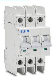
Eaton miniature circuit breaker, current-limiting, 1A, 480Y/277 VAC/96 VDC, 3-pole, D curve, thermal magnetic, 35mm DIN rail mount.
