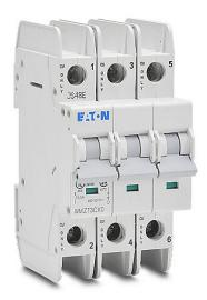
Eaton miniature circuit breaker, current-limiting, 0.5A, 480Y/277 VAC/96 VDC, 3-pole, C curve, thermal magnetic, 35mm DIN rail mount.
