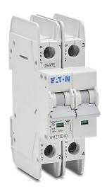
Eaton miniature circuit breaker, current-limiting, 40A, 240 VAC/48 VDC, 2-pole, D curve, thermal magnetic, 35mm DIN rail mount.
