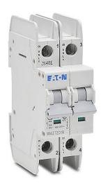
Eaton miniature circuit breaker, current-limiting, 16A, 480Y/277 VAC/96 VDC, 2-pole, D curve, thermal magnetic, 35mm DIN rail mount.
